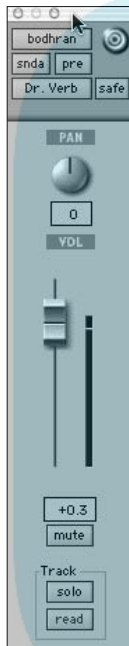
Figure 2-6: Use the Send window to determine send level, mute, pan, and pre- or post-fader settings.
